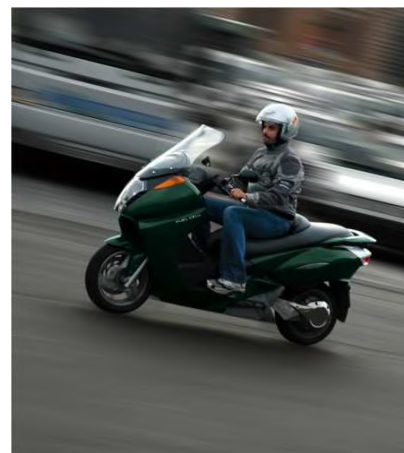
Figure 20.44. Vectrix: 2.75 kWh per 100 km . Photo from www.vectrix.com .
