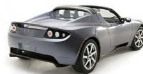
Figure 20.22. Tesla Roadster: 15 kWh per 100 km . www.teslamotors.com .
