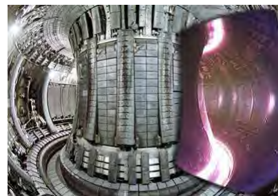
Figure 24.15. The inside of an experimental fusion reactor. Split image showing the JET vacuum vessel with a superimposed image of a JET plasma, taken with an ordinary TV camera. Photo: EFDA-JET.
