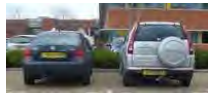
Figure A.5. Power consumed by a car is proportional to its cross-sectional area, during motorway driving, and to its mass, during town driving. Guess which gets better mileage – the VW on the left, or the spaceship?
