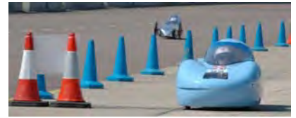
Figure 20.2. Team Crocodile’s eco-car uses 1.3 kWh per 100 km. Photo kindly provided by Team Crocodile. www.teamcrocodile.com
