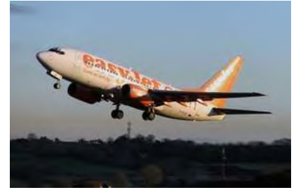
Figure C.11. Boeing 737-700: 30 kWh per 100 passenger-km. Photograph © Tom Collins.
