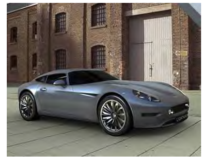
Figure 20.39. Lightning: 11 kWh per 100 km . Photo from www.lightningcarcompany.co.uk.
