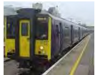
Figure 20.4. This 8-carriage train, at its maximum speed of 100 mph (161 km/h), consumes 1.6 kWh per 100 passenger-km, if full.
