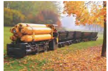
Figure 20.24. Top: A compressed-air tram taking on air and steam in Nantes. Powering the trams of Nantes used 4.4 kg of coal (36 kWh) per vehicle-km, or 115 kWh per 100 p-km , if the trams were full. [5qhvcb] Bottom: A compressed-air locomotive; weight 9.2 t, pressure 175 bar, power 26 kW; photo courtesy of Rüdiger Fach, Rolf-Dieter Reichert, and Frankfurter Feldbahnmuseum.
