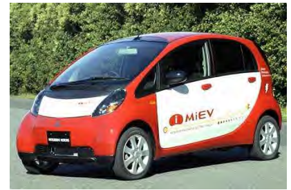
Figure 20.38. The i MiEV from Mitsubishi Motors Corporation. It has a 47 kW motor, weighs 1080 kg, and has a top speed of 130 km/h.
