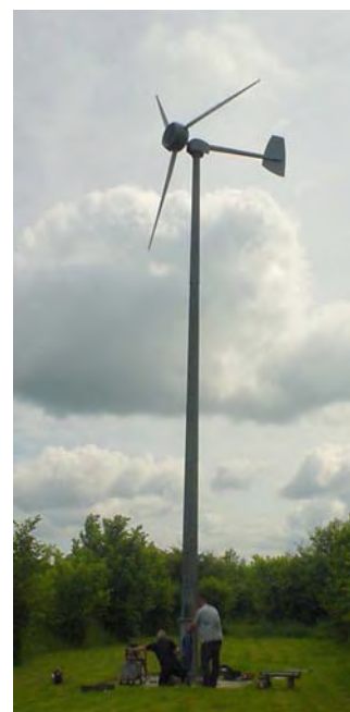
Figure B.10. A 5.5-m diameter Iskra 5 kW turbine [www.iskrawind.com] having its annual check-up. This turbine, located in Hertfordshire (not the windiest of locations in Britain), mounted at a height of 12 m, has an average output of 11 kWh per day. A wind farm of machines with this performance, one per 30 m × 30 m square, would have a power per unit area of 0.5 W/m 2 .
