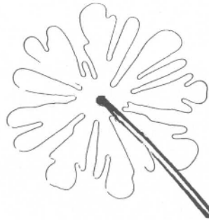
Figure 24.6: Viscous finger pattern in a radial Hele-Shaw cell [152].
