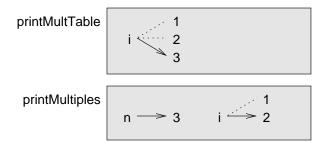
The value of i in printMultTable goes from 1 to 6. In the diagram it happens to be 3. The next time through the loop it will be 4. Each time through the loop, printMultTable calls printMultiples with the current value of i as an argument. That value gets assigned to the parameter n.
