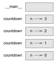
As usual, the top of the stack is the frame for <u>\_\_main\_\_</u>. It is empty because we did not create any variables in <u>\_\_main\_\_</u> or pass any parameters to it.
