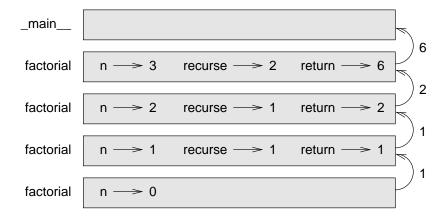
The return values are shown being passed back up the stack. In each frame, the return value is the value of result, which is the product of n and recurse.
