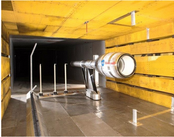
Fig. 10.2 Test section of the NASA Glenn 9- by 15-Foot Low-Speed Wind Tunnel. Image provided by David Stephens, NASA Glenn Research Center.
