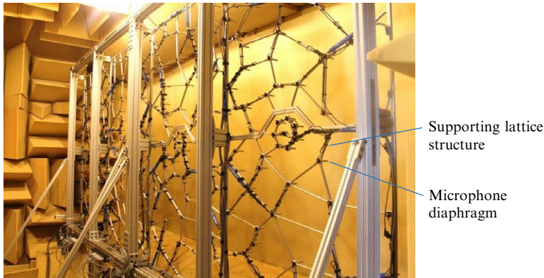
Fig. 10.30 Microphones mounted from behind using an open lattice in the anechoic chamber of a hybrid anechoic wind tunnel.
