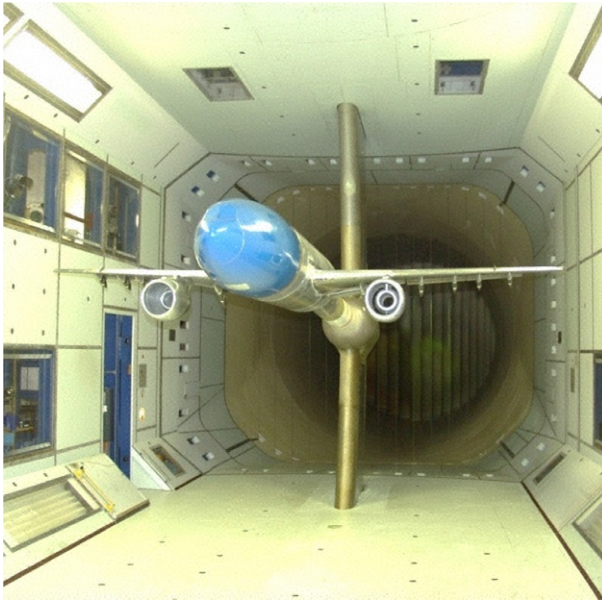
Fig. 10.1 Hard-wall test section of the QinetiQ 5 m wind tunnel at Farnborough, United Kingdom, with a model of an A300 aircraft under test. Image provided by Ian Smith, QinetiQ.
