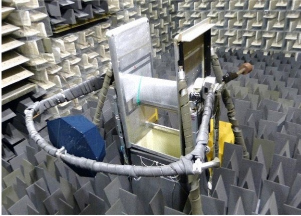
Fig. 10.4 The Quiet Flow Facility at NASA LaRC. Test-section area showing an airfoil model under test and microphone phased array in the foreground. Image provided by Florence Hutcheson and Michael Doty, NASA Langley Research Center.
