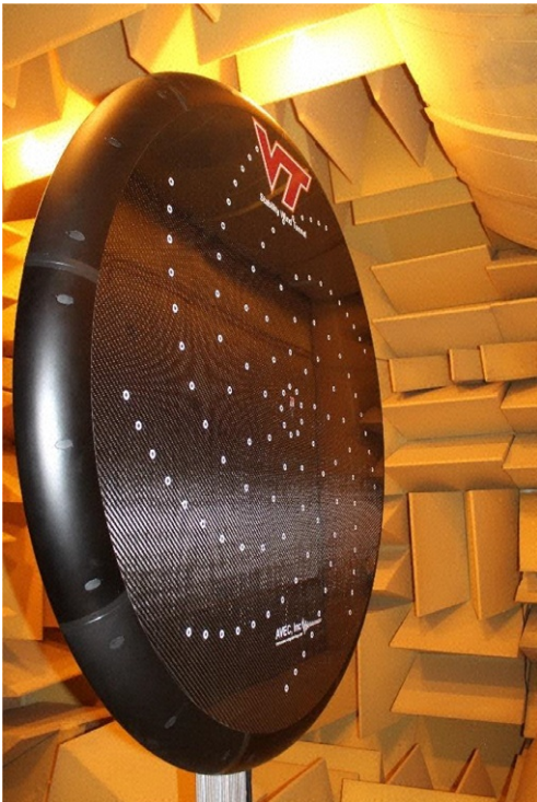
Fig. 10.29 Microphones mounted in a carbon fiber disk to form a 117-microphone phased array.
