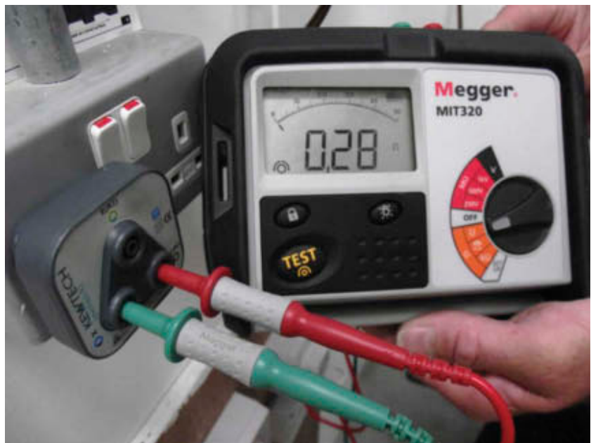
Figure 4.37 Test line to neutral
