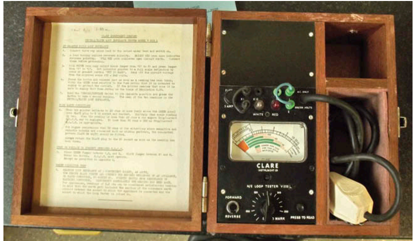
Figure 1.2 Earth fault loop impedance tester
