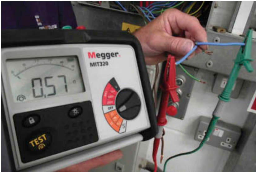
Figure 4.34 Test each end of the neutral conductor
