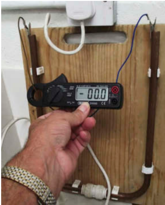
Figure 4.24 Current flow through pipe
