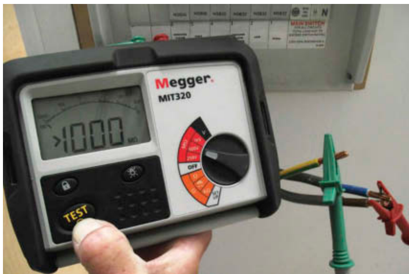
Figure 4.47 Join live conductors and test to earth
