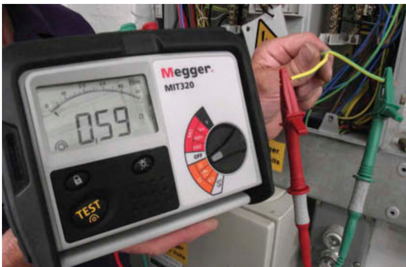
Figure 4.35 Test each end of the CPC
