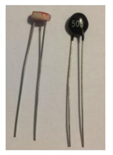
For building sensor hardware, we need 2 resistors, 50k ohm and 10k ohm. If your thermistor is 10k ohm, you should use a resistor with 10k ohm.
