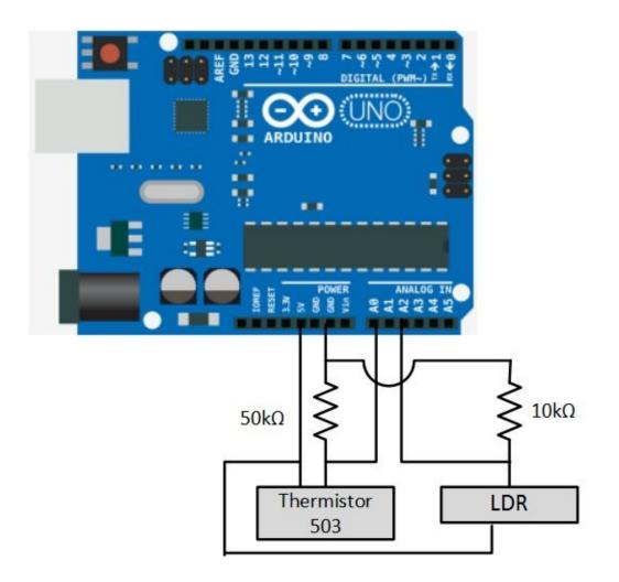
One of sensor pin is connected to 5V Arduino pin. We use a divider approach. Thermistor 503 is attached to the **Analog In** of Arduino, **A0**. Otherwise, LDR is attached to **A2**.
