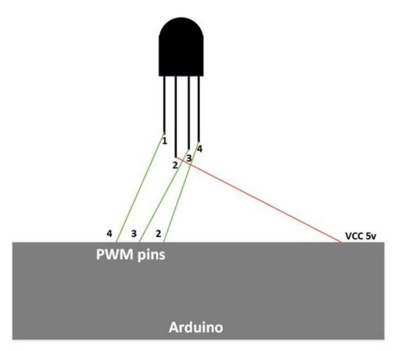
For our testing, we configure the following PWM pins.
