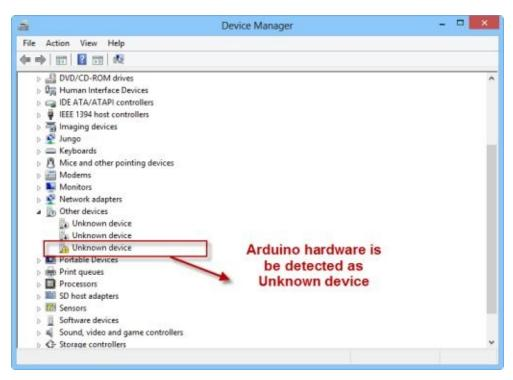
You can update this device driver by navigating hardware driver on the **driver** folder of Arduino software installation folder, for instance **E:\arduino-1.0.2\drivers**.
