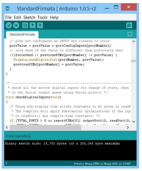
Now you can compile and deploy Firmata Protocol code into your Arduino board. Don't forget to select your Arduino board model and serial port.
