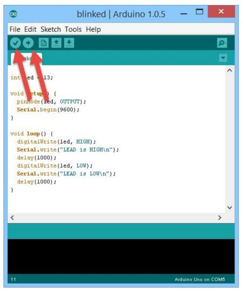
You can check the serial port response using Serial Monitor. Click menu **Tools -> Serial Monitor**. You will see messages from Arduino hardware.
