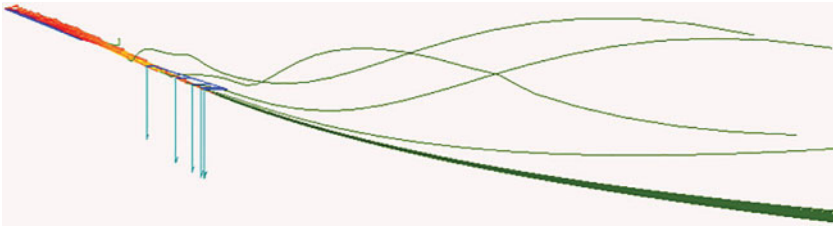
Fig. 5.8 Wing flow slant at a speed of 4 m/s and an angle of 20°.
