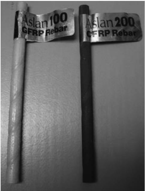
FIGURE 3.7 Carbon and glass FRP bars used in NSM strengthening technology.
