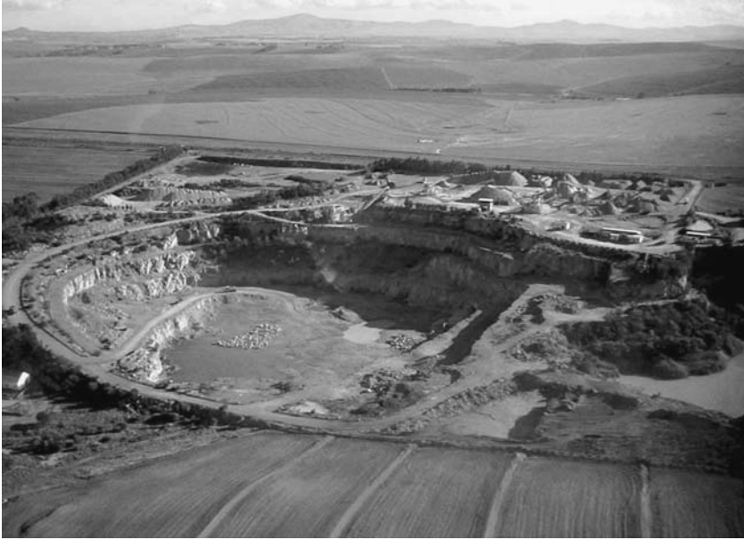
Figure 2.7 Large rock quarry for concrete aggregates (photograph courtesy of ASPASA, via Gill Owens of C&CI).
