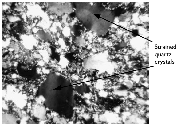
Figure 3.30 Petrographic micrograph of a Cape Peninsula greywacke which is alkali susceptible. Strained quartz grains are shown enclosed in a fine-grained biotite. This type of feature is not detectable without petrographic examination (photomicrograph courtesy of Dr C. Stowe, University of Cape Town).
