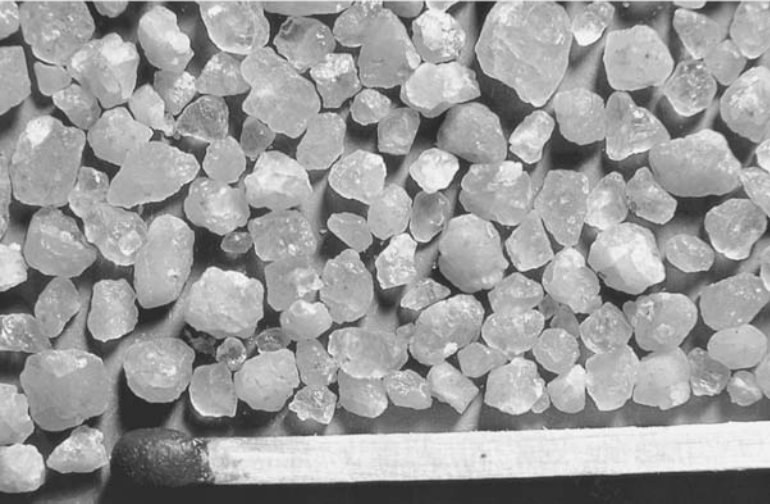
Figure 4.5 Particle shapes of sands and corresponding standard water requirements (SWRs) (scale indicated by matchsticks in Figures 4.5b–f). (a) Clean rounded quartz sand. SWR = 170–180 l/m 3 . (b) Rounded pit sand, good particle shape. SWR = 180–185 l/m 3 . (c) Crushed quartzite sand, reasonable shape. SWR = 200–205 l/m 3 . (d) Crushed quartzite sand, poor shape. SWR = 220–225 l/m 3 . (e) Pit sand, good shape, heavily clay-encrusted. SWR = 220–230 l/m 3 . (f) Weathered granite pit sand. Quartz, decomposed feldspar, and mica. SWR = 220–235 l/m 3 (Photos above Courtesy of Gill Owens, Cement and Concrete Institute).
