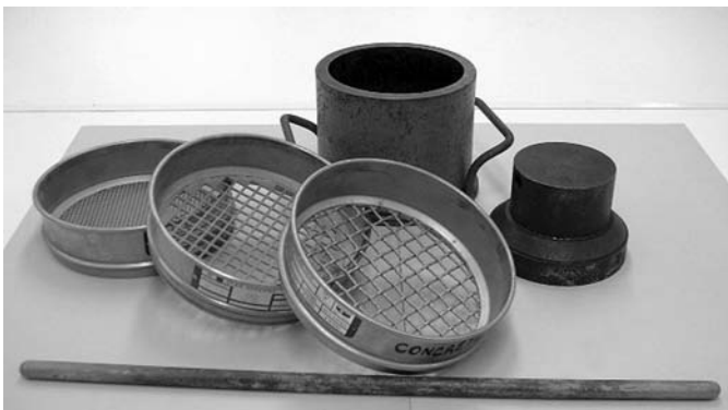
Figure 3.20 Apparatus for 10% FACT and ACV tests. Note confining steel cylinder and plunger, compacting rod, and different sieve sizes.
