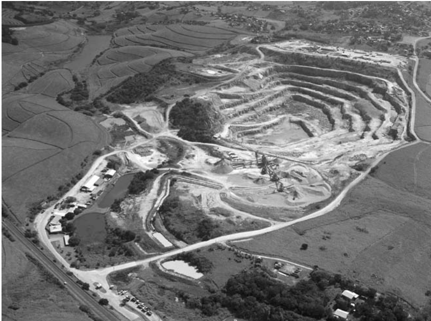
Figure 1.3 Large regional quarry showing various environmental aspects: remote from built-up areas; dam in upper LH corner; large visual impact; containment of operation. Long-term plan to return site to agriculture and recreation uses (photograph courtesy of ASPASA, via Gill Owens of C&CI).
