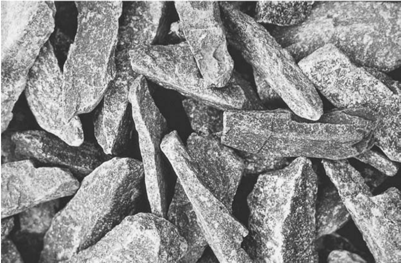
Figure 4.4 (a) Well-rounded aggregate showing good packing. Void content \approx 33\% . (b) Angular and poorly shaped aggregate showing poor packing and particle interlock. Void content \approx 45\% . (Photo Courtesy of Gill Owens, Cement and Concrete Institute). Maximum aggregate size for both aggregates approximately 25 mm.
