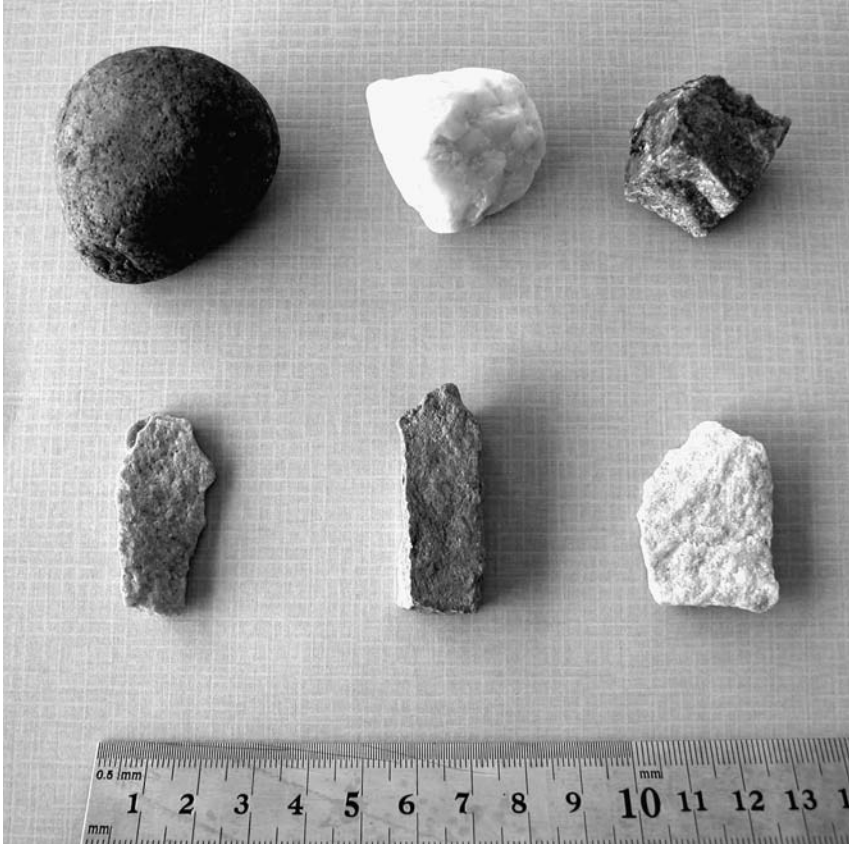
Figure 3.6 Illustrations of particle shapes. Shapes (according to BS 812: Part 102: 1989) are, clockwise from top left: Rounded, Irregular, Angular, Flaky, Elongated, Flaky and Elongated.
