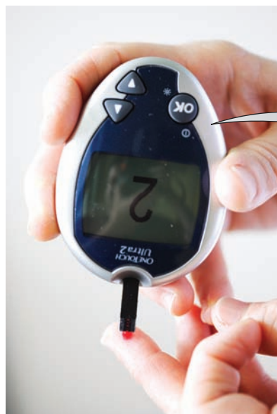
Figure 14.13 Biosensor for blood glucose testing
