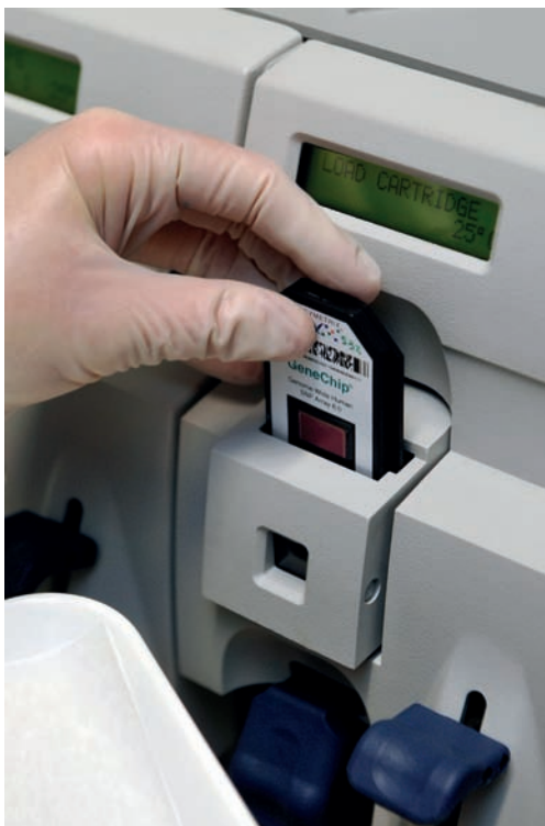
Figure 19.10 Microarray analysis machine with microarray being inserted
