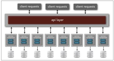
Figure 3-5. Microservices architecture topology
