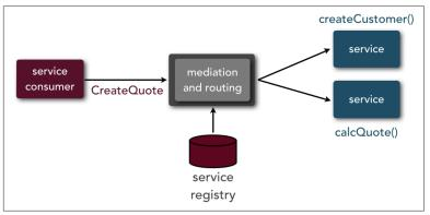
Figure 3-9. Mediation and routing capability
