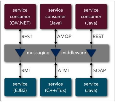
Figure 4-2. Protocol-agnostic heterogeneous interoperability
