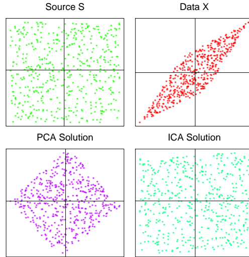
FIGURE 14.38. Mixtures of independent uniform random variables. The upper left panel shows 500 realizations from the two independent uniform sources, the upper right panel their mixed versions. The lower two panels show the PCA and ICA solutions, respectively.
