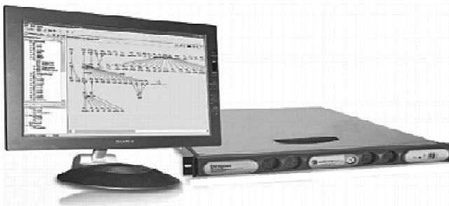
Figure 7.5 Administration control console of an appliance-based IDPS. Enterasys Dragon Network IDS Appliance (Fast Ethernet). (From NIST, Guide to Intrusion Detection and Prevention Systems, http://csrc.nist.gov/publications/nistpubs/800-94/SP800-94.pdf .)
