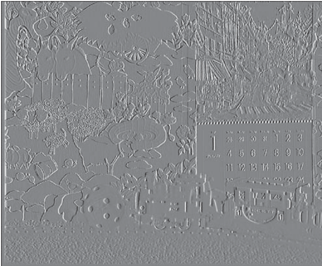
Figure 3.22 One-dimensional DPCM difference picture for first picture in “Mobile and Calendar” sequence (shifted by 128 and scaled by 2).
