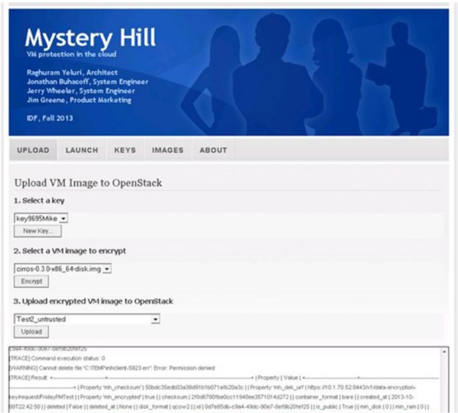
Figure 8-7. Selecting and binding a virtual machine image to an encryption key
