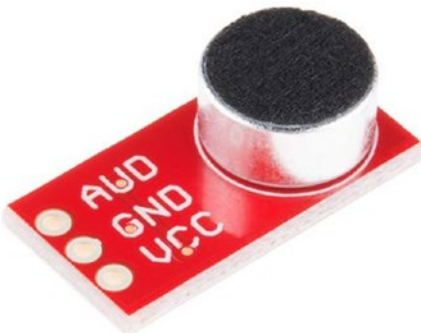
Figure 3-3. SparkFun Electret Microphone Breakout from SparkFun
