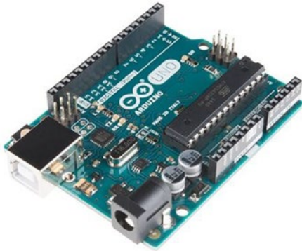
Figure 1-2. Arduino UNO board from Arduino LLC
