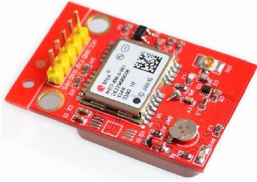
Figure 5-37. GPS Module with U-blox device
