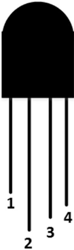
Figure 3-10. RGB LED pin layout
