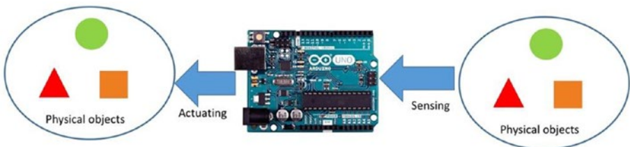
Figure 3-1. Sensing and actuating on Arduino board
