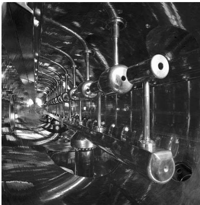
12. The particle accelerator used at the Institute for Heavy Ion Research (GSI) in Darmstadt, Germany, for fusing atomic nuclei to make new superheavy elements. The GSI team have used this equipment to make all the elements from 107 to 112
