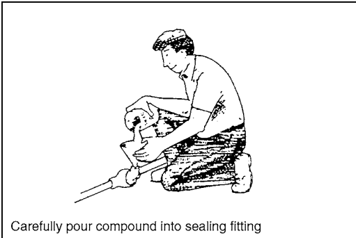
FIGURE 9-4. Carefully pour compound into sealing fitting.
