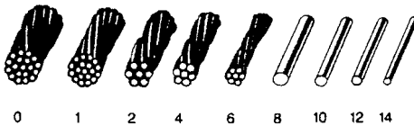
FIGURE 8-1. Common sizes of wire.
