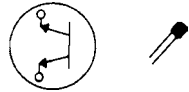
FIGURE 15-3. A diac, or diode AC switch, is used with triacs and SCRs.
