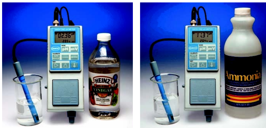
FIGURE 14.7 pH meters are used to measure acidity.
