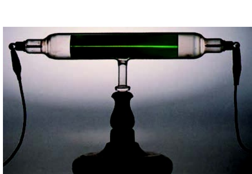
FIGURE 2.7 A cathode-ray tube. The fast-moving electrons excite the gas in the tube, causing a glow between the electrodes. The green color in the photo is due to the response of the screen (coated with zinc sulfide) to the electron beam.
