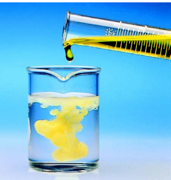
FIGURE 4.13 When yellow aqueous potassium chromate is added to a colorless barium nitrate solution, yellow barium chromate precipitates.
