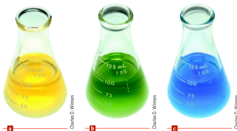
FIGURE 15.7 (a) Yellow acid form of bromthymol blue; (b) a greenish tint is seen when the solution contains 1 part blue and 10 parts yellow; (c) blue basic form.
