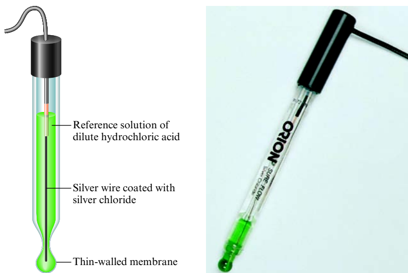
FIGURE 18.12 A glass electrode contains a reference solution of dilute hydrochloric acid in contact with a thin glass membrane in which a silver wire coated with silver chloride has been embedded. When the electrode is dipped into a solution containing \text{H}^+ ions, the electrode potential is determined by the difference in [\text{H}^+] between the two solutions.
