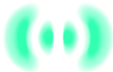
FIGURE 7.16 A cross section of the electron probability distribution for a 3p orbital.
