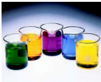
▲ Various chromium compounds dissolved in water. From left to right: \text{CrCl}_2 , \text{K}_2\text{Cr}_2\text{O}_7 , \text{Cr}(\text{NO}_3)_3 , \text{CrCl}_3 , \text{K}_2\text{CrO}_4 .
