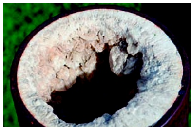
FIGURE 11.9 A pipe with accumulated mineral deposits. The cross section clearly indicates the reduction in pipe capacity.
