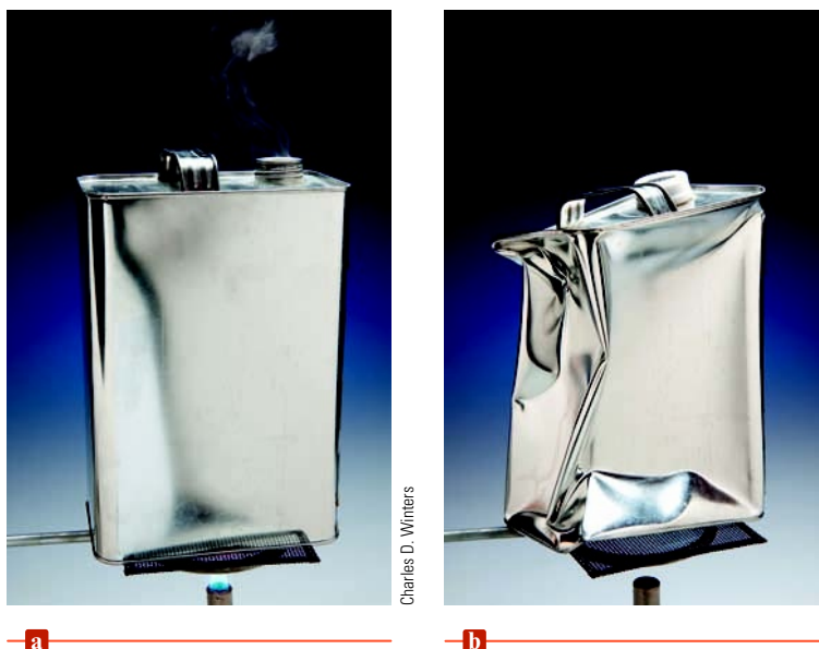
FIGURE 5.1 The pressure exerted by the gases in the atmosphere can be demonstrated by boiling water in a large metal can ( a ) and then turning off the heat and sealing the can. As the can cools, the water vapor condenses, lowering the gas pressure inside the can. This causes the can to crumple ( b ).
