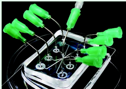
A microfluidic lab on a chip. Stainless steel needles inserted into the device serve as access points for fluids.
