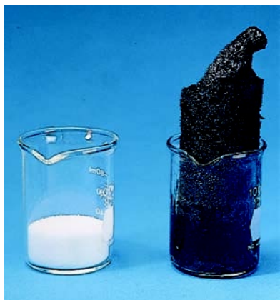
FIGURE 20.24 The reaction of \text{H}_2\text{SO}_4 with sucrose (left) to produce a blackened column of carbon (right).
