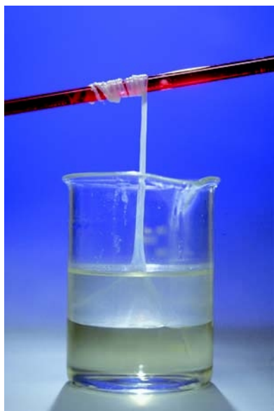
FIGURE 22.16 The reaction to form nylon can be carried out at the interface of two immiscible liquid layers in a beaker. The bottom layer contains adipic acid dissolved in \text{CCl}_4 , and the top layer contains hexamethylenediamine dissolved in water. A molecule of \text{HCl} is formed as each C—N bond forms.
