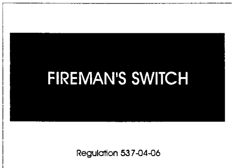
Figure 9.19: Fireman's switch notice
