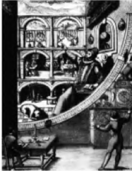
Figure 4.3. A mural depicting Tycho Brahe's quadrant that had a radius of 2 m. Tycho is shown both at the right edge as an observer and also as the large figure at the centre of the mural.
