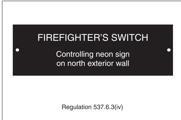
Figure 9.20 Remote fireman's switch notice
