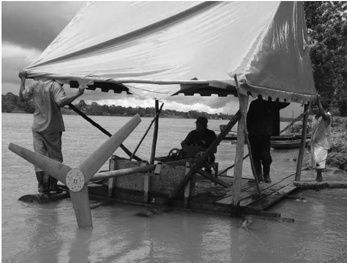
FIGURE 12.9 River current turbine. (From Practical Action Latin America (Soluciones Prácticas).)
