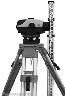
FIGURE 3.1 A level machine mounted on a tripod and staff.
