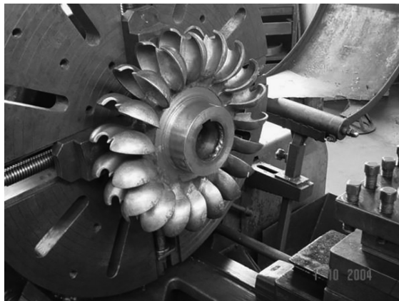
FIGURE 2.25 A 100-kW Pelton turbine in a workshop, Nepal.
