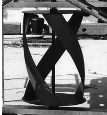
FIGURE 12.13 Gorlov helical turbine. (From http://www.gcktechnology.com/ )
