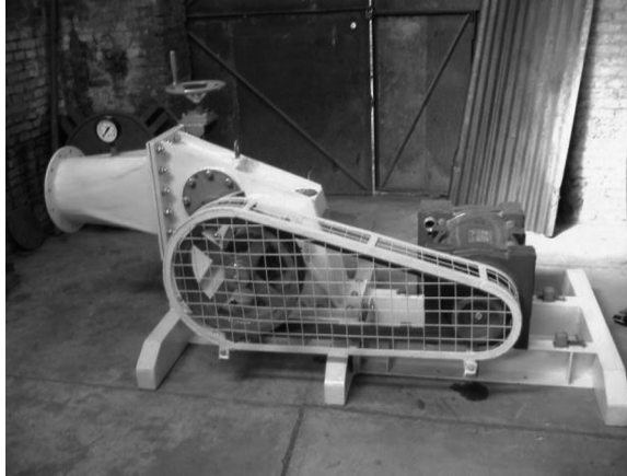
FIGURE 2.26 An induction generator coupled with a cross-flow micro hydro turbine, Nepal.
