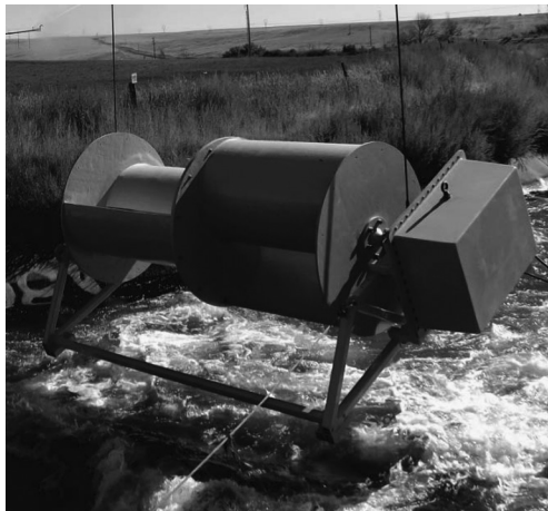
FIGURE 12.11 Horizontal axis Savonius design. (Hydrovolt C-12 Canal Turbine.)
