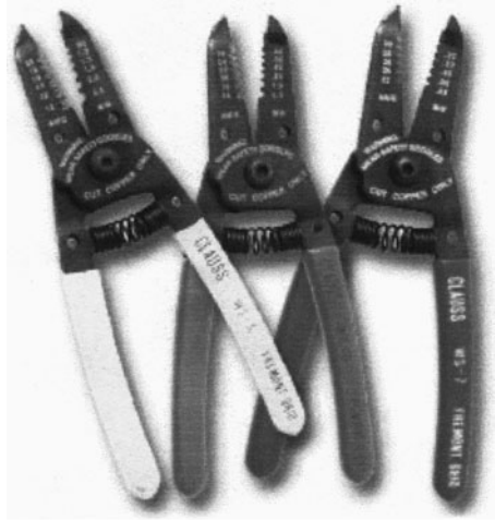
FIGURE 11-14. (J) Wire strippers and cutters. (K) Wire strippers.
