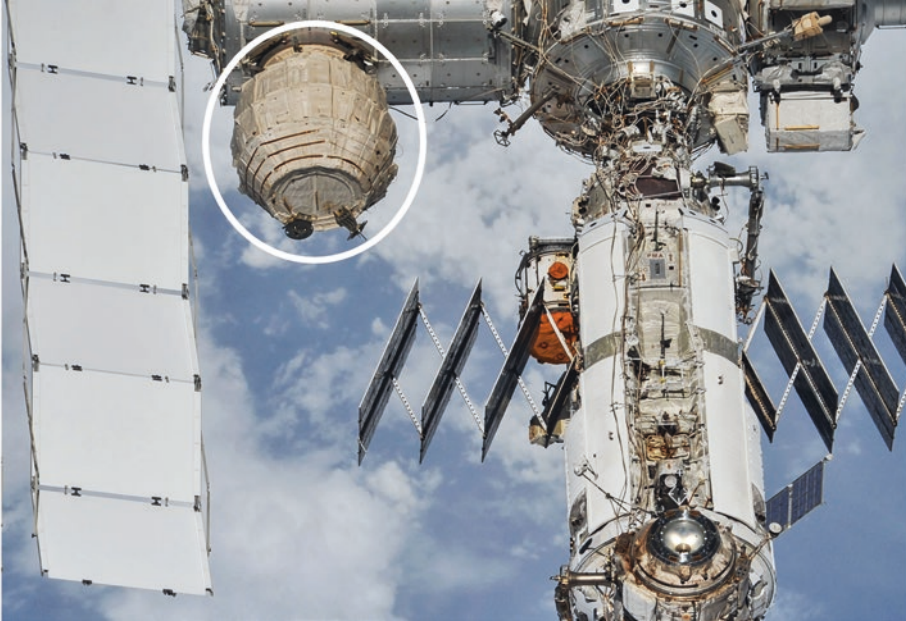
Figure 6.19 The Bigelow Expandable Activity Module (BEAM) in its current position on the International Space Station (highlighted with a white circle). Although small in comparison with other modules, it is the forerunner of much larger inflatables that will expand our capability to live and work in space.
