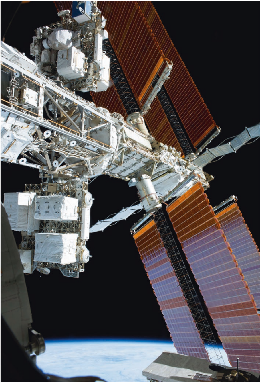
Figure 6.17 Two platforms for storage of spare parts placed either side of the truss structure.
