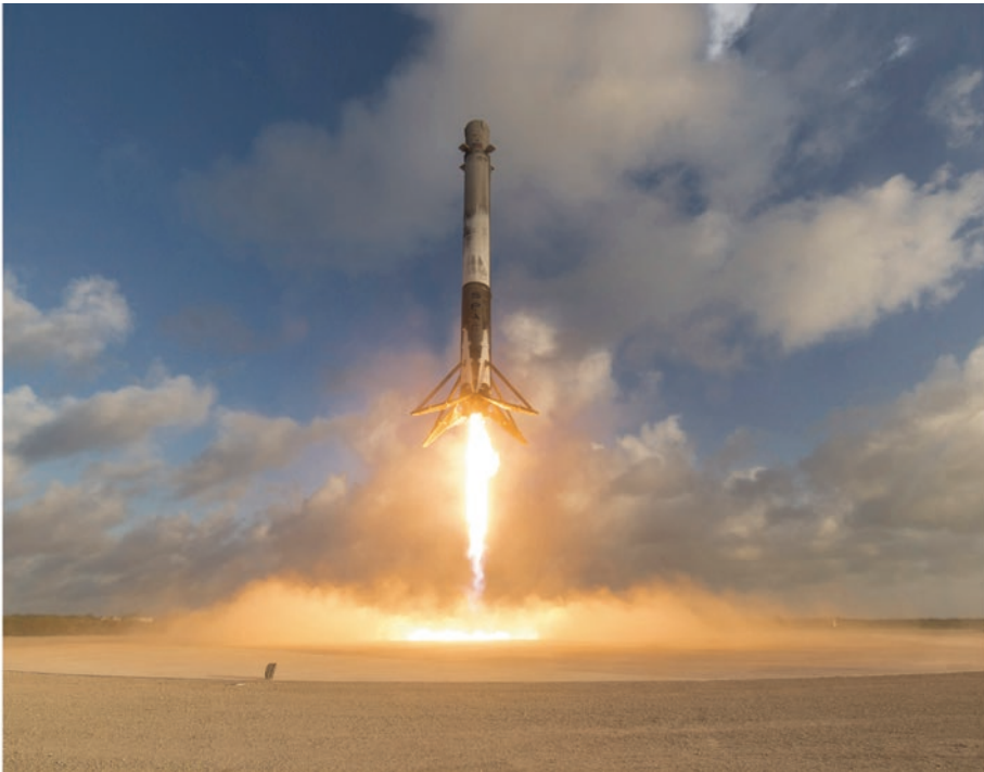
Figure 7.1 A SpaceX Falcon 9 first stage is about to land after another successful launch.
