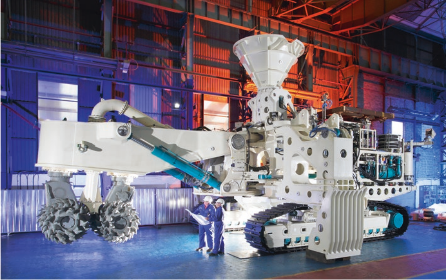
Figure 7.9 The Nautilus Minerals Auxiliary Cutter (used with permission from Nautilus Minerals, Inc.)
