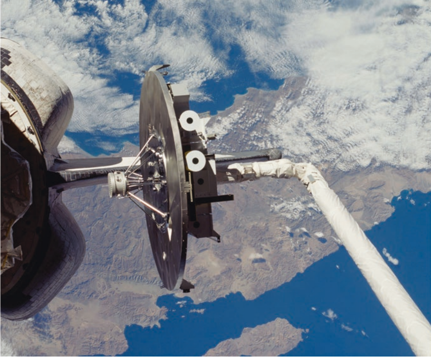
Figure 5.11 The Wake Shield Facility is removed from the Space Shuttle's cargo bay. The source cell apparatus is visible on the wake side of the platform.
