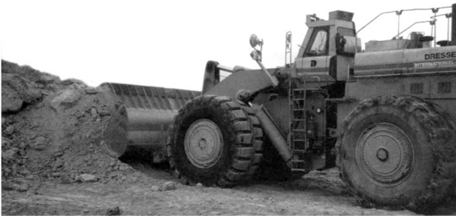
Figure 3.4 A good muck pile is well-fragmented and largely contained in one heap. Loading would be much more time consuming if the rock were widely dispersed, as might be the case using conventional blasting in a low-gravity environment and the absence of air resistance. The loading machine must have sufficient traction (created by friction and weight) to push the loading bucket into the muck pile.
