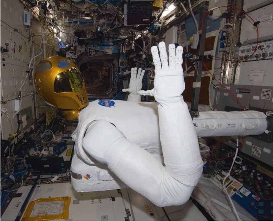
Figure 6.14 The dexterous humanoid Robonaut is now a permanent resident of the International Space Station.
