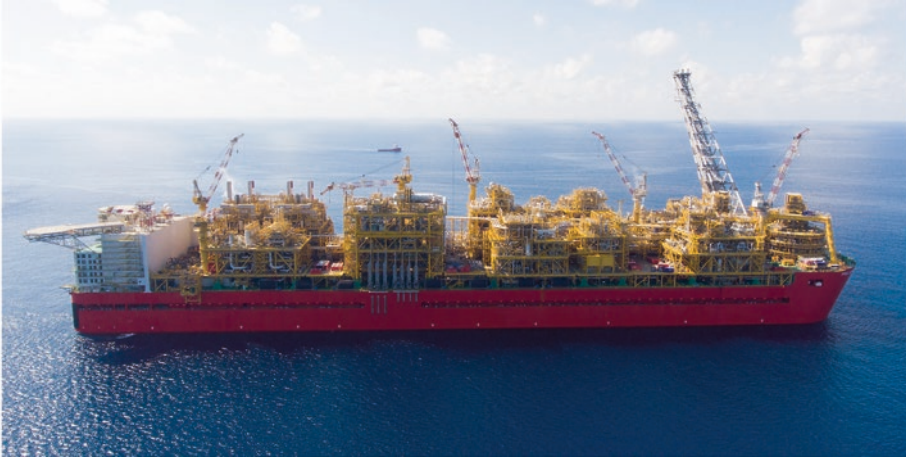
Figure 7.13 An overview of the Prelude floating liquefied natural gas (FLNG) facility, illustrating its sheer size and complexity.
