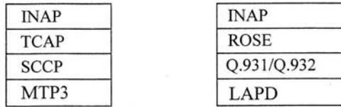
Figure 18.4-1 INAP protocol stacks.
