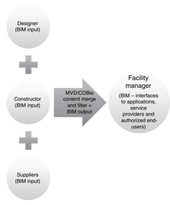
Fig. 15.2 BIM information and data exchange.
