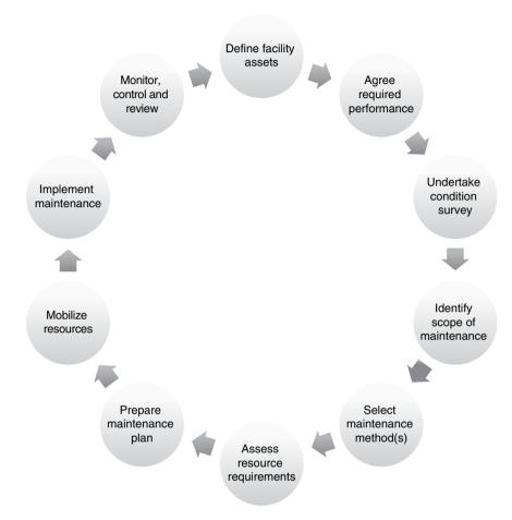
Fig. 12.1 The maintenance process.
