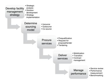
Fig. 1.2 A basic plan for facility management.
