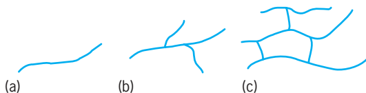
Fig. 1. Polymer chains. (a) Linear polymer chain. (b) Branched polymer chain. (c) Cross-linked polymer chain.
