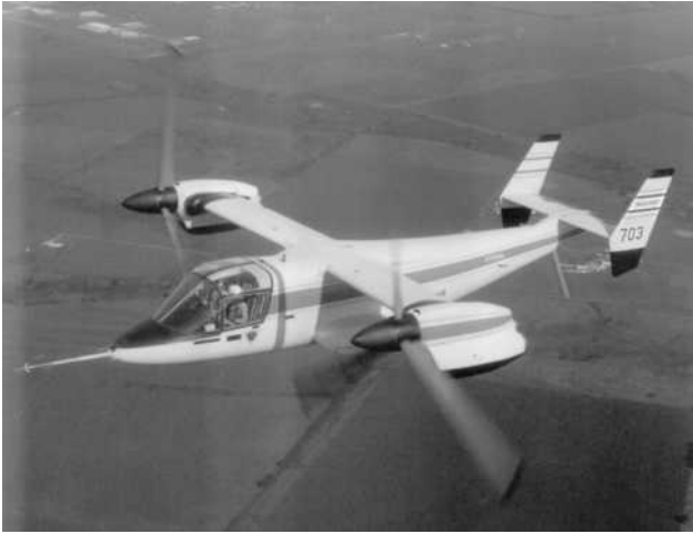
Fig. 1. NASA-Army-Bell XV-15 in airplane configuration after conversion from helicopter mode. (Bell Helicopter Textron)
