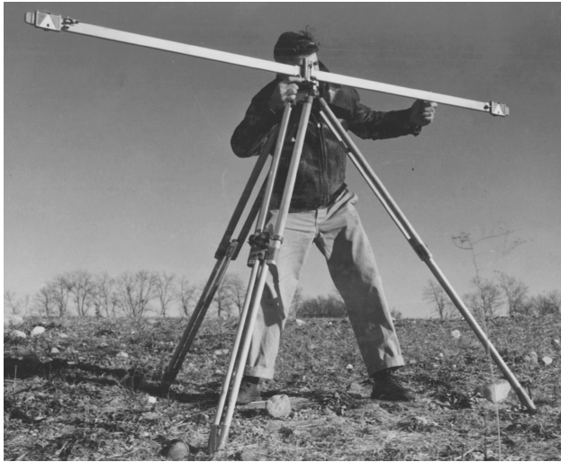
Fig. 1. Subtense bar. (Lockwood, Kessler, and Bartlett Inc.)
