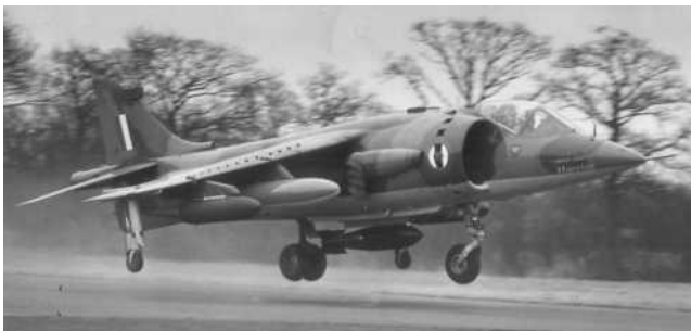
Fig. 3. Harrier fighter aircraft, manufactured by Hawker Siddeley, now British Aerospace, and McDonnell Douglas. Close ground support and reconnaissance are provided through use of vectored-thrust turbofans.
