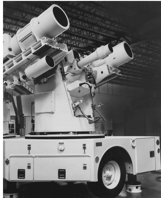
KINETO Model 433 Tracking Mount shown with 100- and 200-in. focal-length (2.5- and 5.1-m) motion picture cameras, both with 12-in. (30-cm) aperture, and a 40–240-in. focal-length (1.0–6.1-m), 6-in.-aperture (15-cm) television camera. The fourth platform is reserved for either a laser ranger or a thermal imaging system. (Contraves Goerz Corp.)
