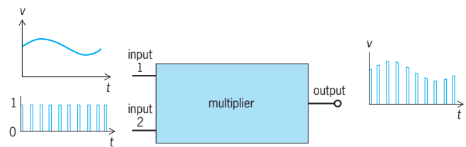
Fig. 1. Pulse-amplitude modulation by means of a multiplier circuit.
