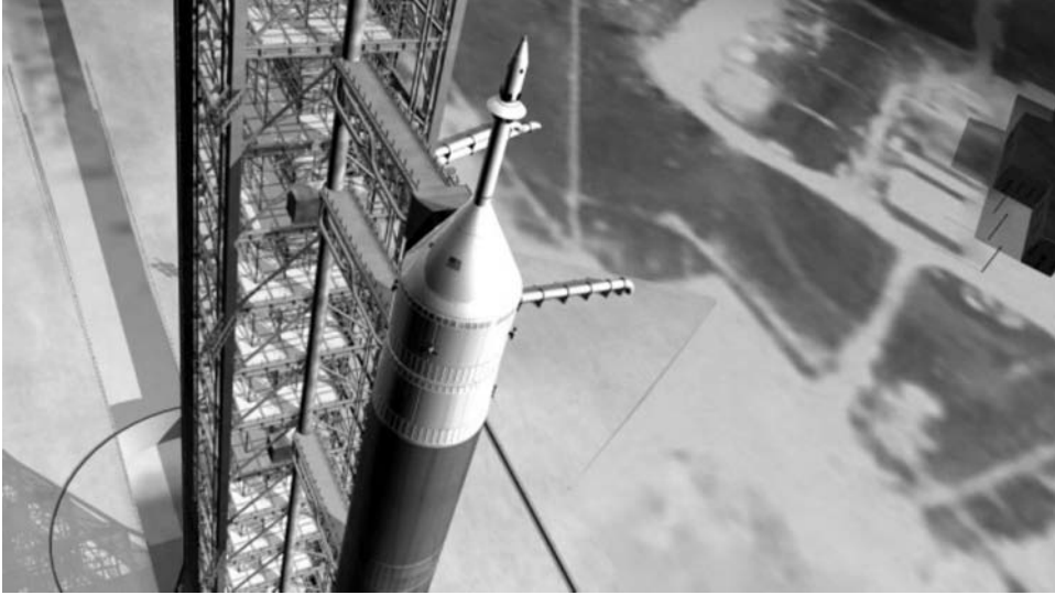
Artist's impression of the Ares launch vehicle on the pad with the Orion manned spacecraft and Launch Escape System in place.
