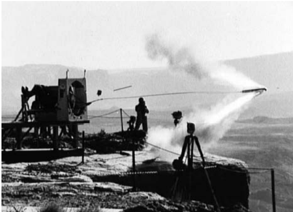
Leaving the Orbiter (top). Testing the tractor rocket escape system (bottom).
