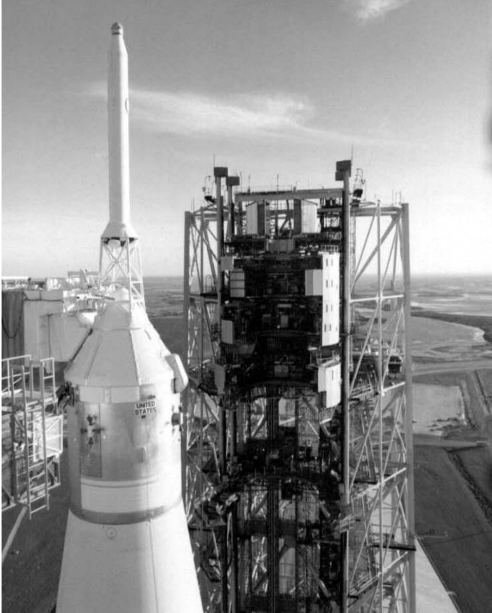
Launch Escape System mounted on top of the Apollo 8 stack.
