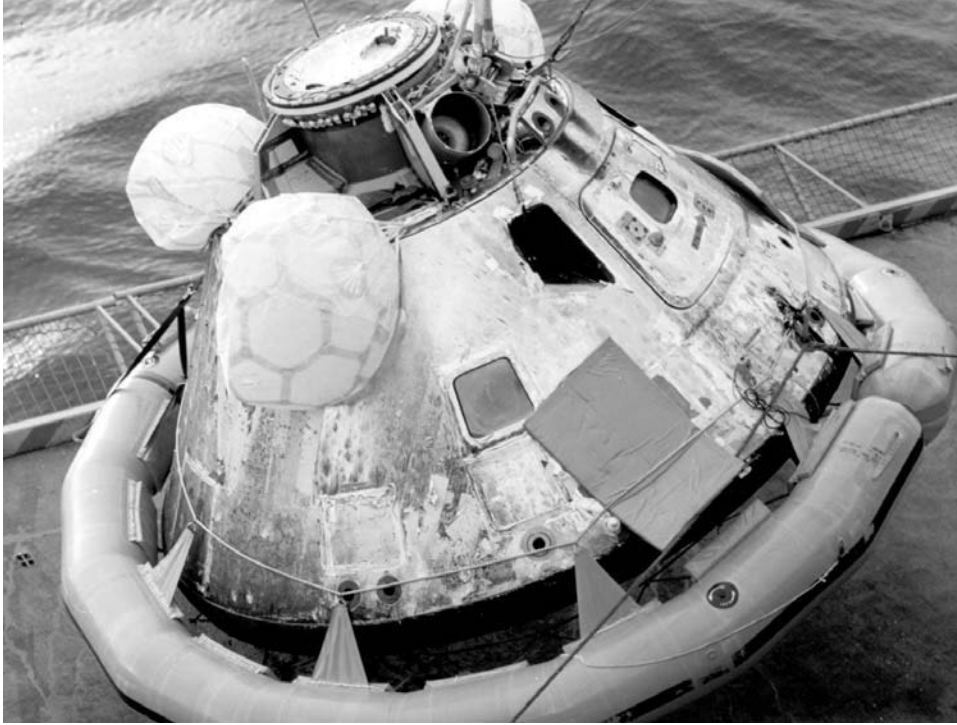
Apollo flotation collar and self-righting balloons.
