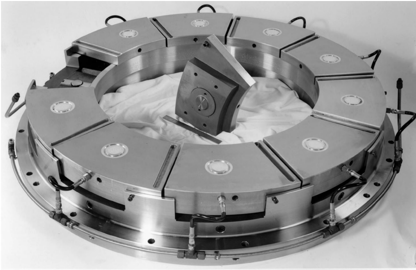
Figure 7.12 Pivoted pad thrust bearing with leading edge oil feed groove and oil lift pockets for low-friction starting. (Courtesy Kingsbury, Inc.)
