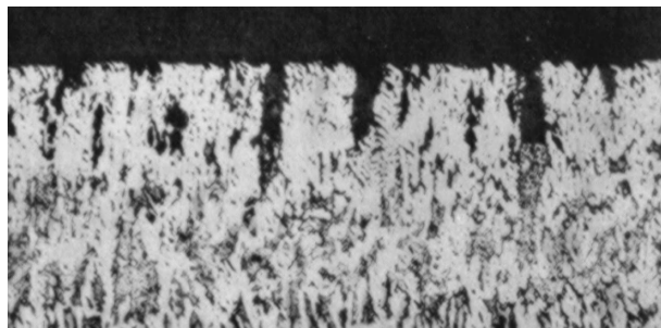
Figure 17.10 Lead corroded from copper–lead bearing by oxidized oil. (Burgess, 1953)
