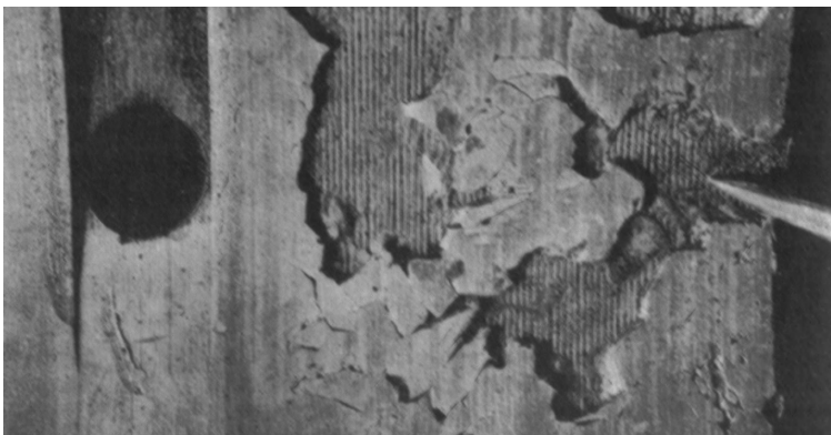
Figure 17.7 Fatigue failure of babbitt bearing. (Burgess, 1953)
