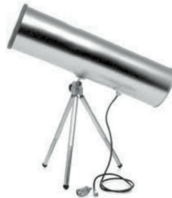
Homemade directional antenna
