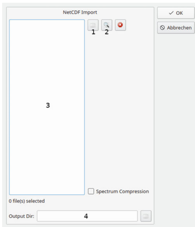
Fig. 2 The netCDF import dialog. Files for import can be selected directly (1) or searched for recursively in a folder (2). The selected files will appear on the left (3). Optionally, a different output directory can be selected (4)
