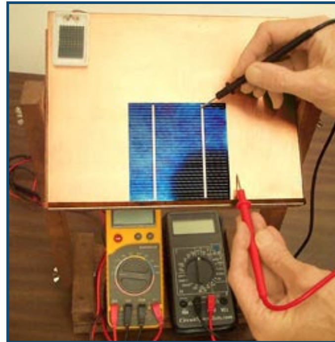
Stand for testing solar cells
