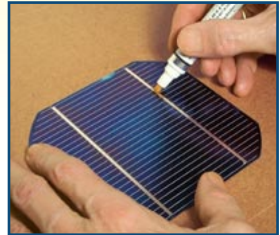
Applying flux with a pen before soldering tab ribbon to the cells
