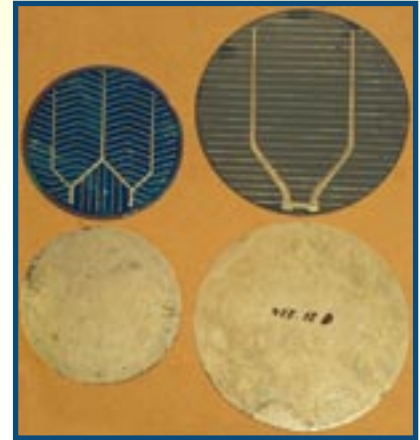
Above, older style cells, with solder covering the backs; below, newer cell with six solder spots on the back.
