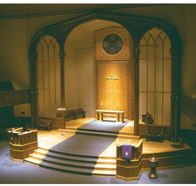
Plate 8-1 (far left) Modern Cathedral. The altar and throne are illuminated for television using focal lighting. Other focal lighting layers illuminate the large hanging sculpture. Wallwashing illuminates wood panels behind sanctuary. No decorative lighting. Photo: Luminae Souter Lighting Design
