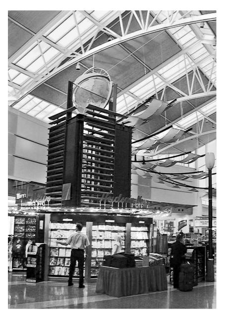
Daylighted Airport Terminal with Most of the Electric Lighting Extinguished
