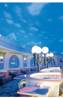
**Plate 6-1** (far left) Layers used to make artificial sky and day/night effect. Uplight using only 4100K white lamps, all other sources off. *Photo: J. Benya*
