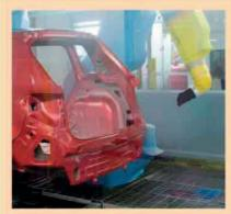
**Paint robots** at this Volkswagen factory help reduce employee costs, and can be programed to use the minimum amount of paint required.
