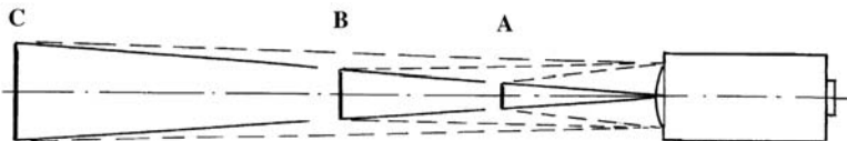
Figure 4.11 Schematic demonstration of the path of light for an automatic optical pyrometer. At a given distance A the required minimum target size is moderate (e.g., 5 mm dia.) and the cone of free sight (dashed lines) widens towards the lens opening. At the distance B the required target diameter is doubled, and at C it is quadrupled, with a correspondingly large required cone of free sight.
