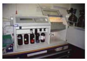
Figure 17.3 Automated instrument for the extraction of DNA from blood samples of  $5-20 \,\mathrm{ml}$  volumes
