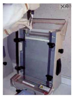
Figure 17.11 Loading PCR-ampilified DNA onto an SSCP/heteroduplex gel
