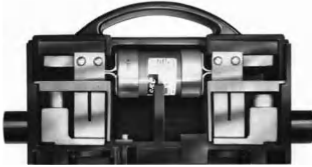
Fig. 16.9 Sectioned fuse-holder showing how extensive shrouding of live parts is achieved.
