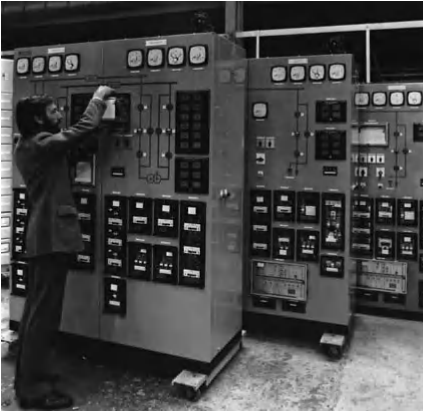
Fig. 2.11 Final adjustments being made on a control and instrumentation panel for Equador. Note the semaphores on the panel front ( Arcontrol Ltd ).
