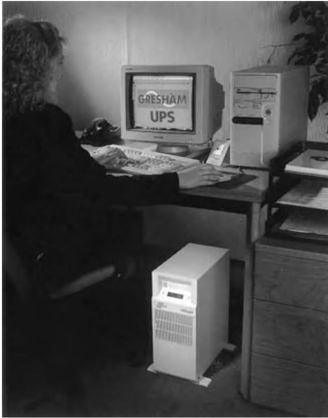
Fig. 6.19 Modern UPS systems need to be designed for the office environment. They need to be compact, easy to use, quiet and stylishly designed. The unit shown is a 500 VA on-line UPS, which at full load provides 15 minutes back-up power – enough time to complete important tasks, save data and perform an orderly shutdown. Battery extension packs can be added to extend the duty period up to several hours running time.
