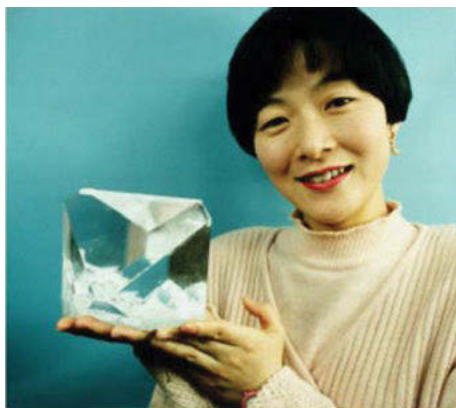
Figure 6.3.3: Photograph of large CLBO crystal with dimensions of 14 \times 11 \times 11 \text{ cm}^3 for three weeks growth. Reprinted from Mori Y, Kuroda I, Nakajima S, Sasaki T, Nakai S. New nonlinear optical crystal: Cesium lithium borate. Appl Phys Lett 1995,67,1818–20, with the permission of AIP Publishing.
