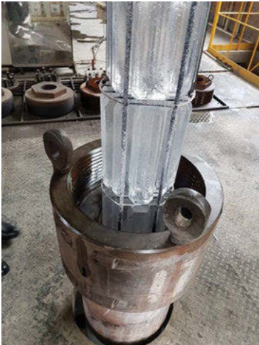
Figure 6.7.11: Quartz crystals harvested after hydrothermal crystal growth.
