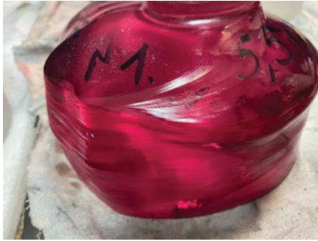
Figure 6.7.7: Ti-sapphire grown by the Kyropoulos method, diameter 250 mm.
