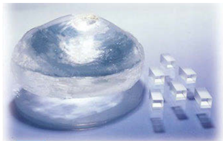
Figure 8.6.4: Single crystal of \beta -BBO. With courtesy and permission from Castech ( https://gb.castech.com/product/106.html ).
