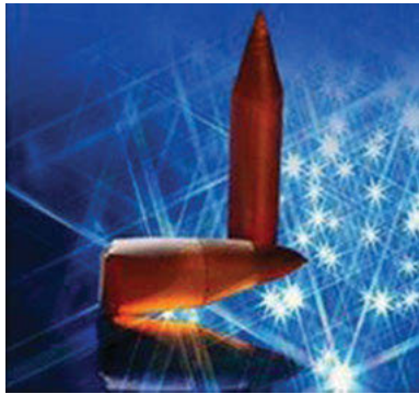
Figure 8.6.41: Photo of large as-grown \text{LiInS}_2 crystals with a diameter of 16 \text{ mm} and a length of 50 \text{ mm} . Reproduced with permission from ref. [193]. Copyright 2014. American Chemical Society.
