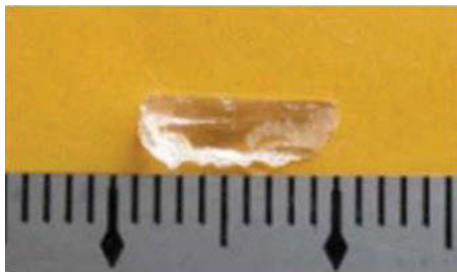
Figure 8.6.13: Photograph of K_3B_6O_{10}Cl . Reproduced with permission from ref. [73]. Copyright 2011 American Chemical Society.
