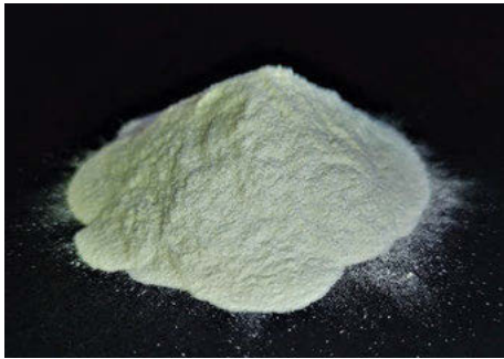
Figure 8.2.3: Photographic image of a \text{Pr}^{3+} activated upconverter under standard indoor illumination (Photograph by Patrick Pues).
