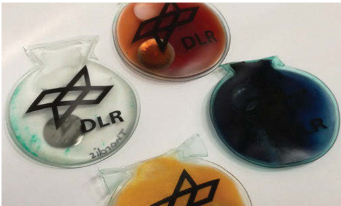
Figure 5.6.2: Pocket warmer with sodium acetate trihydrate in a plastic bag. Bending the metal clip triggers rapid crystallization and heat release.
