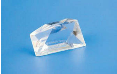
Figure 8.6.7: Photograph of a large CsLiB 6 O 10 crystal produced by CASTECH, Inc. With courtesy and permission from Castech ( https://gb.castech.com/product/CLBO-%E6%99%B6%E4%BD%93-108.html ).
