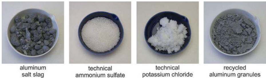
Figure 6.4.3: Fractions of the salt slag processing. The samples were kindly provided by K + S. Fotos by Thomas Fickenscher.
