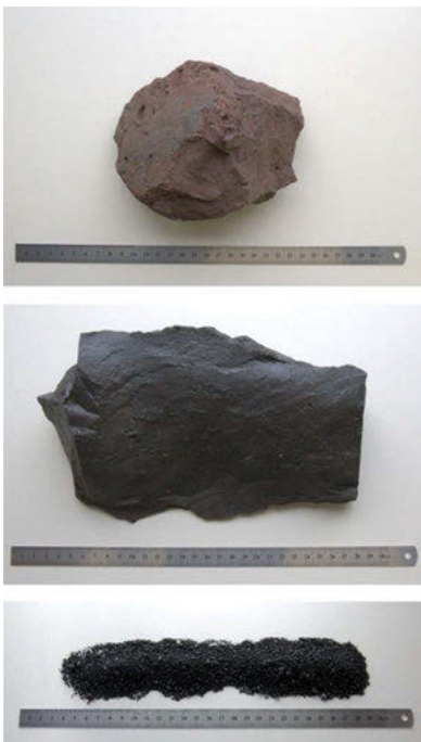
Figure 6.4.4: (top) Copper slag of an anode furnace, (middle) converter slag and (bottom) granulated iron silicate slag. The samples were kindly provided by Aurubis AG. Fotos by Thomas Fickenscher.
