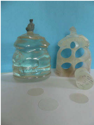
Figure 6.7.9: Kyropoulos sapphire-boule core drilled and cut into wafers for use as a wafer in blue emitting LED production.
