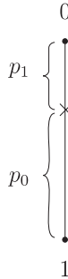
Fig. 3.2 A probabilistic classical bit. Here the probabilities p_0 and p_1 of the bit being 0 and 1, respectively, are represented by the position of a point on the line segment between the points representing 0 and 1.
