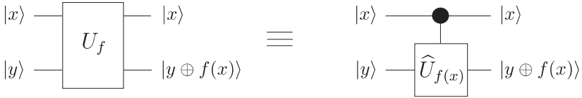
Fig. 6.6 The 2-qubit gate U_f : |x\rangle|y\rangle \mapsto |x\rangle|y \oplus f(x)\rangle can be thought of as a 1-qubit gate \hat{U}_{f(x)} acting on the second qubit, controlled by the first qubit.
