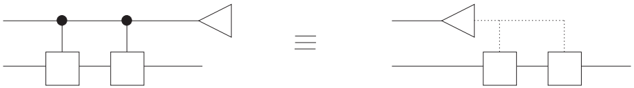
Fig. 4.7 Suppose that at some point in a computation there is some qubit that will only be used as a control qubit in subsequent controlled- U_b operations before being discarded. The same result is obtained if one measures the qubit in the computational basis and then classically controls the U_b gates.
