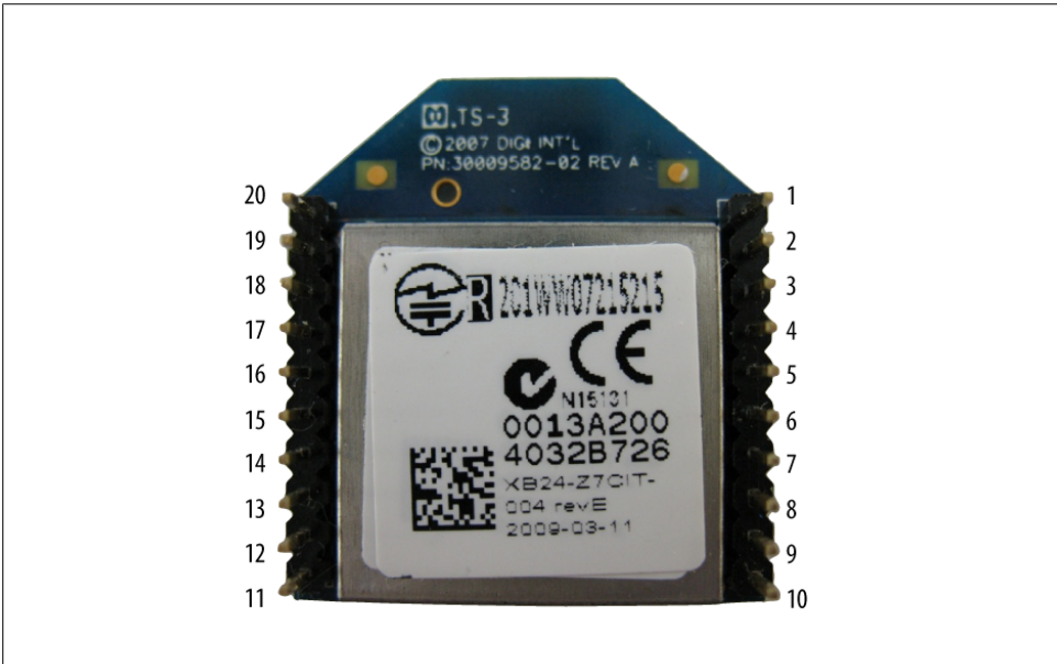
Figure 1-12. XBee physical pin numbering, back view
