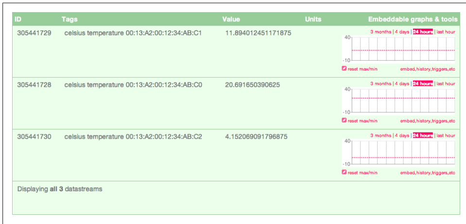
Figure 8-8. Pachube data streams are at the bottom of the Output screen for each Feed. In this case the ID created is the decimal version of the XBee's 64-bit ID, so that each ID is unique.
