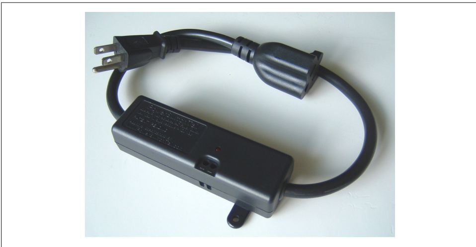
Figure 6-3. PowerSwitch Tail 5 V relay for A/C loads
