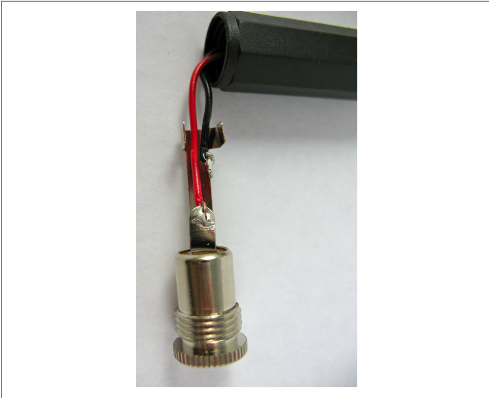
Figure 5-5. Power jack with wiring soldered in place
