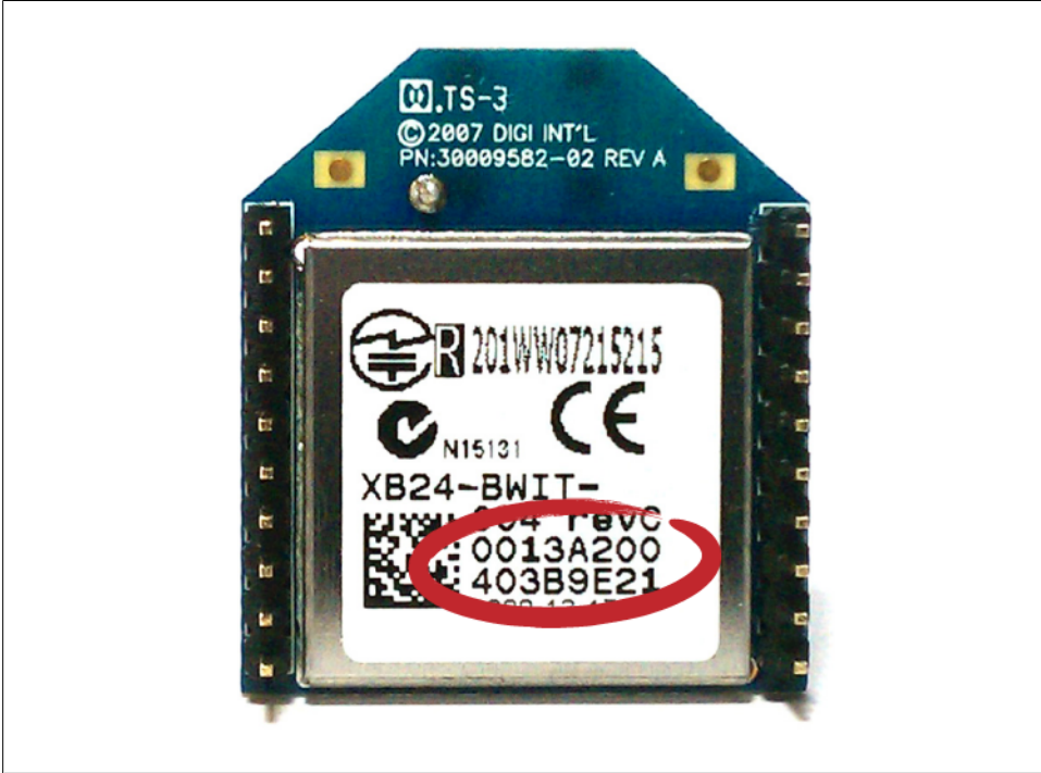
Figure 2-22. Back of XBee showing 64-bit address
