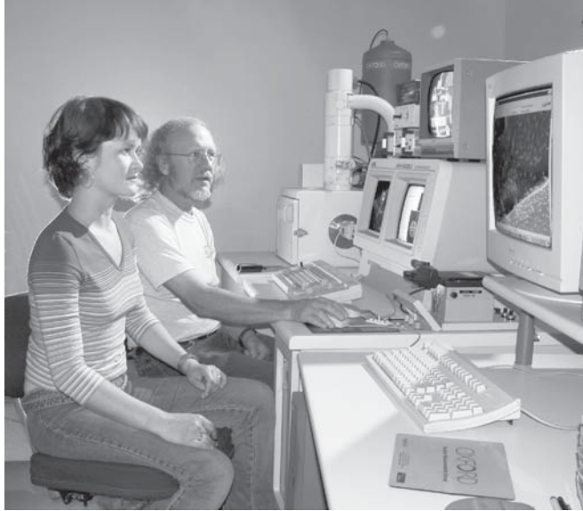
Figure 5.8. Scanning electron microscope equipped with X-ray dispersive spectroscopy. (Image courtesy of Kenneth Ingham.)
