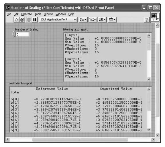
Figure L5-14: Fixed-point analysis using DFD toolkit (no scaling).
