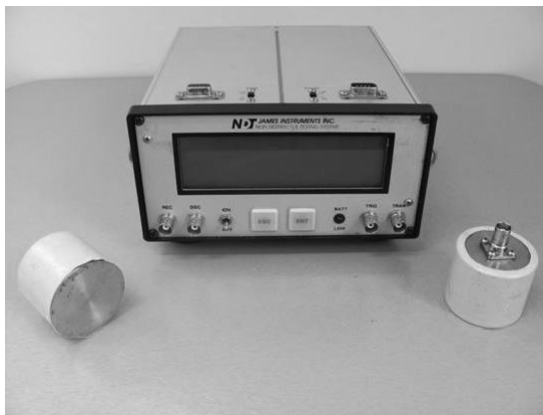
FIGURE 12.12 Photograph of ultrasonic pulse velocity equipment.
