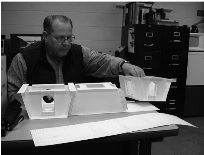
FIGURE 2.4 During project planning, a fabricator may make scale models of the components to be fabricated to help him work out the best fabrication approach.
