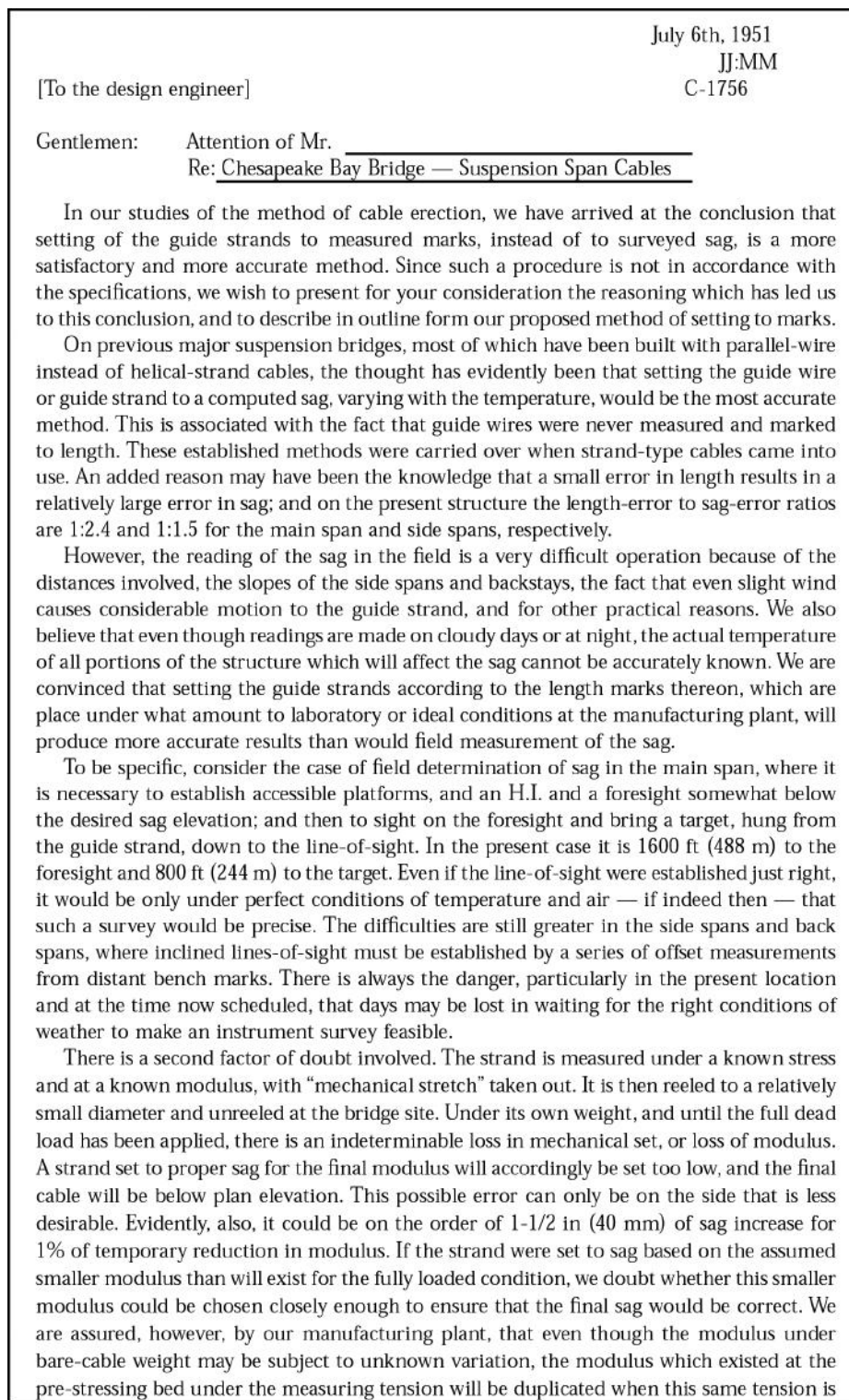
FIGURE 1.7 Setting cable guide strands to marks.
