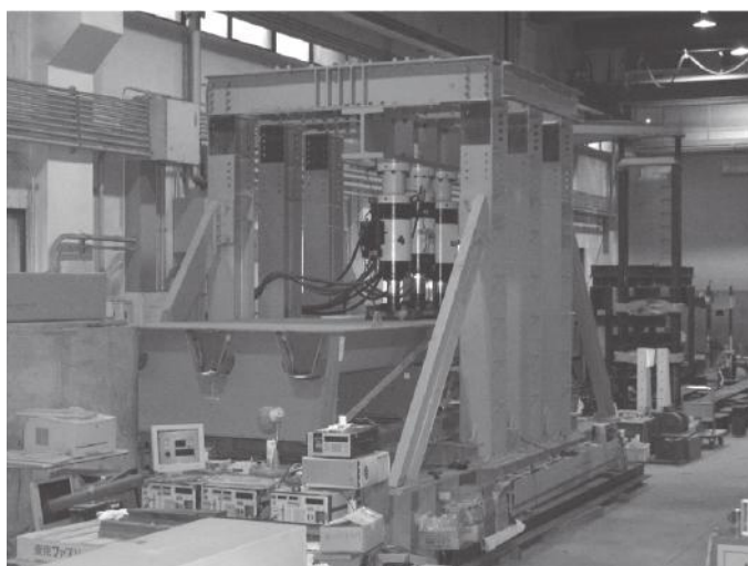
FIGURE 17.73 Three-jack system to simulate moving loads.
