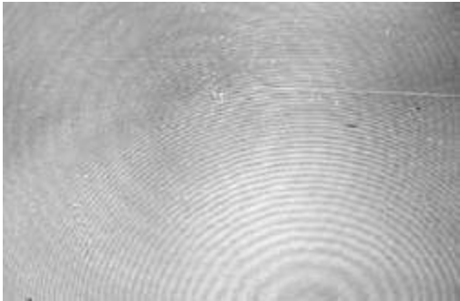
Figure 15: A waveform interference pattern that holds the information that transforms into a hologram.
