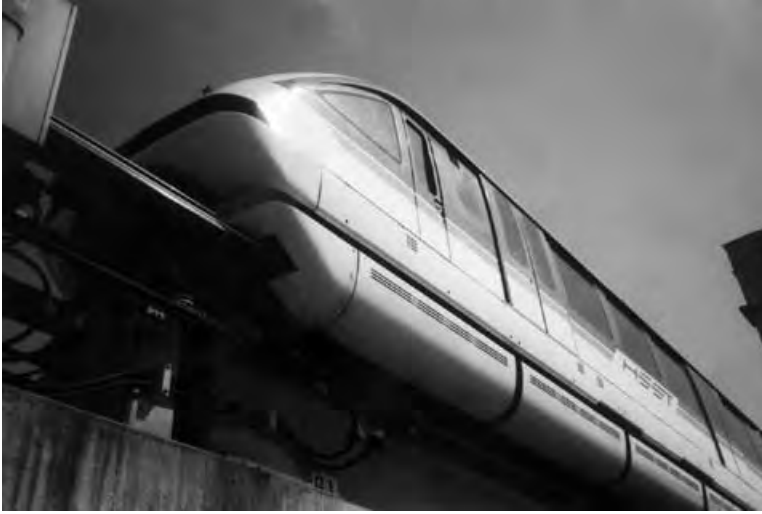
FIGURE 6.4 Magnetically levitated rigid body (HSST MagLev prototype vehicle, 1998, Nagoya, Japan).
