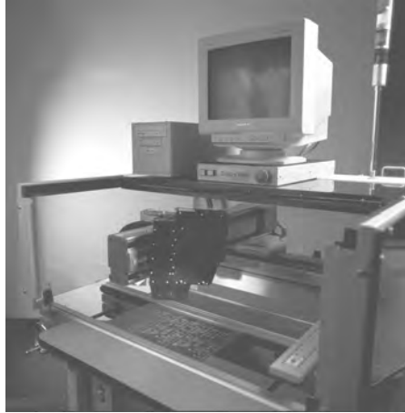
FIGURE 13.1 An optical inspection system for printed circuit boards. (Used by permission © CyberOptics Corporation 2001, all rights reserved.)
