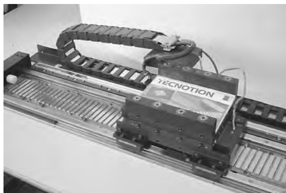
FIGURE 12.24 Linear motor. The magnets that cause the cogging are clearly visible.
