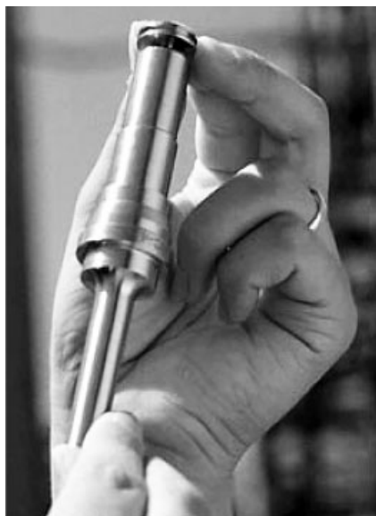
Fig. 9-4 Today the BASIL™ process is run in a small jet reactor that has a capacity of 690\,000\text{ kg m}^{-3}\text{ h}^{-1} . © BASF Aktiengesellschaft 2002.
