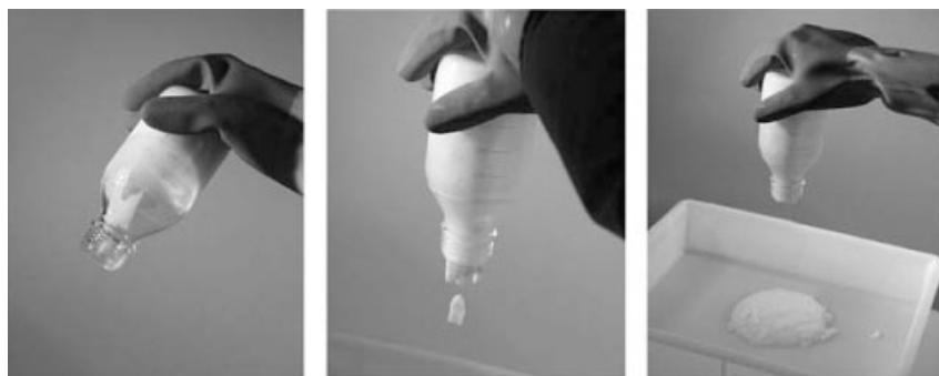
Fig. 9-2 The slurry that is formed when a tertiary amine is used as an acid scavenger. © BASF Aktiengesellschaft 2003.
