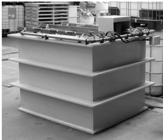
Fig. 9-9 1200 L demonstrator module for electropolishing. © Scionix 2005.
