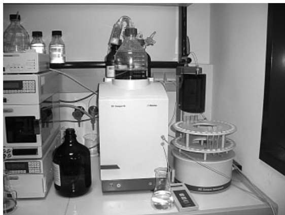
Fig. 2.2-2 Ion chromatography – the method of choice for the quantification of ionic impurities in ionic liquids.
