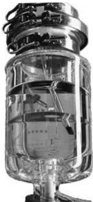
Fig. 9-3 The BASIL™ process. After the reaction two clear liquid phases are obtained - the upper being the pure product the lower being the ionic liquid [HMIM]Cl. © BASF Aktiengesellschaft 2002.
