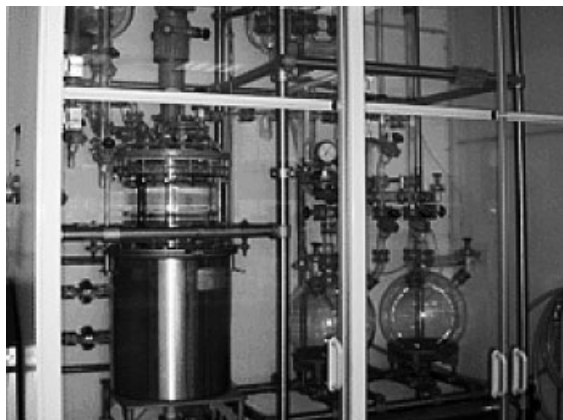
Fig. 2.2-3 100 liter reactor for ionic liquid production at Solvent Innovation.
