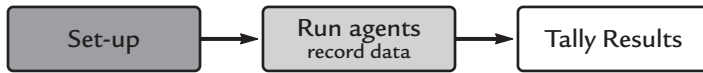
Figure 11–3 The overall test is divided into three parts. The setup part describes the test environment, number of concurrently running test agents, and behavior of each agent based on a user archetype. The second part actually runs the agents and records the results to a log file. The third part analyzes the recorded results and presents the findings.
