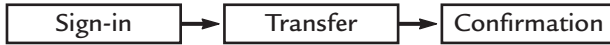
Figure 6-1 The customer sees three pages in the browser when transferring funds. However, behind the scenes, actually six HTTP transactions take place.
