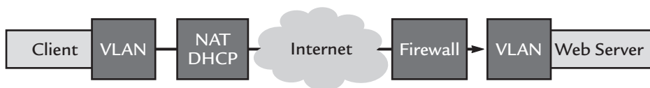
Figure 10–3 Software at the client and server devices to encrypt data communicated over a Web infrastructure forms a VPN.
