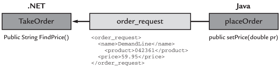
Figure 9–1 The Java placeOrder function makes a SOAP request to the TakeOrder method of the published Web service.
