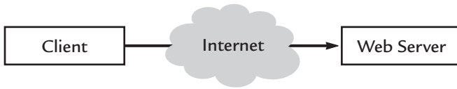
Figure 10-1 Basic network connections for open Web sites put the client in direct connection to the server.
