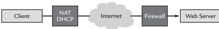
Figure 10-2 Routers that provide Network Address Translation and firewall functions also provide a form of security that protects the client machine from being hacked.
