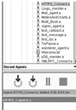
Figure 5–4 The Execution panel is below the Explorer panel and controls running a test agent on the local machine, running a test agent on a distributed set of TestNetwork nodes, pausing a running agent, and stopping a test agent.
