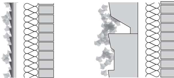
19.10 Living wall systems (based on planter boxes and based on felt layers) without the exterior masonry for a total integration of the greening concept.
