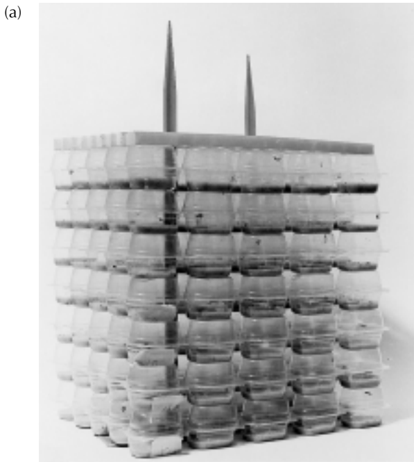
Fig. 1A.1. (and opposite) Dietary larval rearing trays for bioassays of B. thuringiensis . (a) Disposable gel trays for bioassays with 3rd-instar larvae. Each cell is filled with 1 g of diet. The lid is an empty gel tray placed upside down. (b) A 24-well tray. Well dimensions: 15 mm diameter \times 17 mm depth. (c) A grid of 21 cells each sized 13 \times 13 \times 6 mm cut from a fluorescent light shading, made of plastic (cell size: 11 mm 2 ; wall thickness: 2.5 mm) and fitted into a 9-cm disposable Petri dish.
